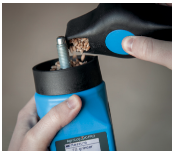
Put the sample in the grinder and grind. The sample size is measured out in the built-in measuring cup.
