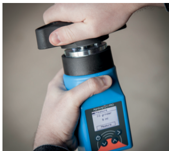
Press the top button and read the moisture content directly from the display.
