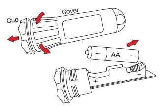
**3.** Open the sensor cover and remove the battery if it has been already inserted. Don't twist the cup, to avoid cable damage.
