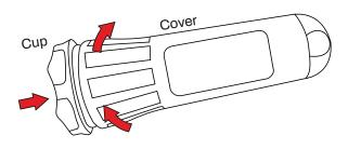
**6.** After successful pairing, close the sensor by screwing the sensor cover back on the cup.
