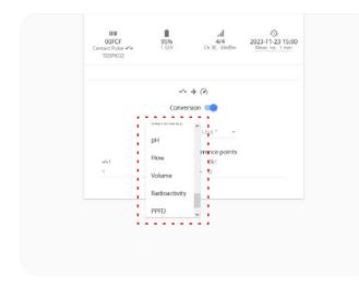
**9.** To do that switch the Conversion on, and use the drop-down menu to choose a predefined Dimension and unit.
