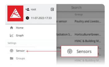
**1.** In the user interface of the base station accessed through **WiFi-IP** in a web browser, go to **@ Sensors**.
