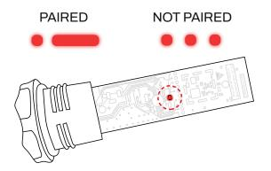
**5.** Successful pairing is confirmed by one short and one long LED light flash and takes up to 30 seconds. Failed pairing is indicated by three short flashes.
