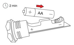
**4.** The 2 min timer indicates the window to insert the battery in the sensor. Correct battery type for each sensor is indicated in its datasheet.
