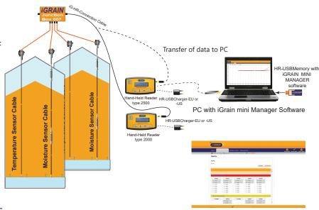
one by one. Model 2500 has the same basic functions as model 2000; but it can also connect to a PC. With the iGrain Mini Manager software installed on the PC for storing downloaded sensor data the PC will be able to show the readings and trend curves.
